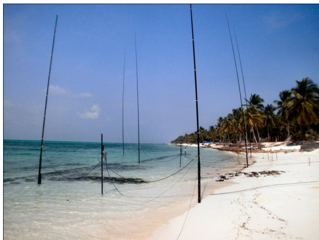
VU7AG's 30m, 40m and 80m phased arrays on Agatti
