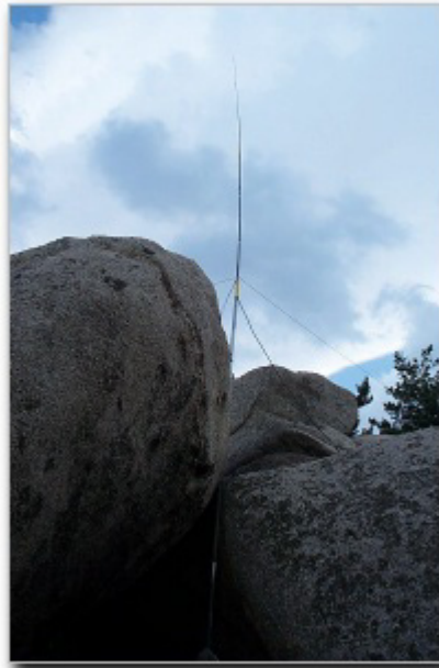
Home made vertical 20m mono band-we used to first day contact to I1JQJ & IK1ADH
